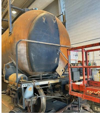
The headshield is being applied to the tank car. (Photo credit: Tyler Yates, GATX)
