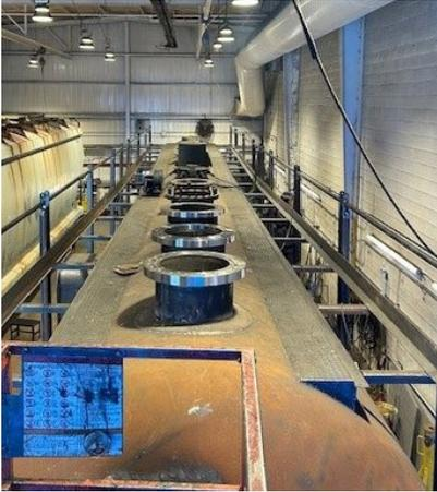
The construction team has made great progress, and all top display housings have been applied. (Photo credit: Tyler Yates, GATX)
