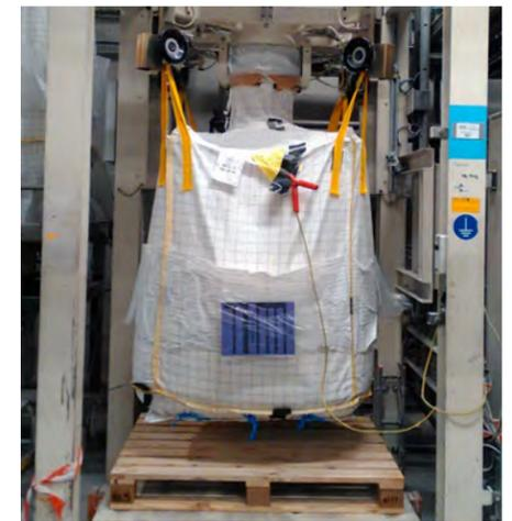
Figure 6. A Flexible Intermediate Bulk Container (FIBC) containing a dry solid chemical. Note the yellow lifting straps and the external grounding attachment.
