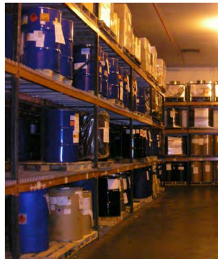
Figure 1. Bulk storage of chemicals in a warehouse in portable drums (steel, plastic, fiber) and metal totes. When needed, the chemicals are moved on pallets by hand truck or forklift to the chemical processing area.
